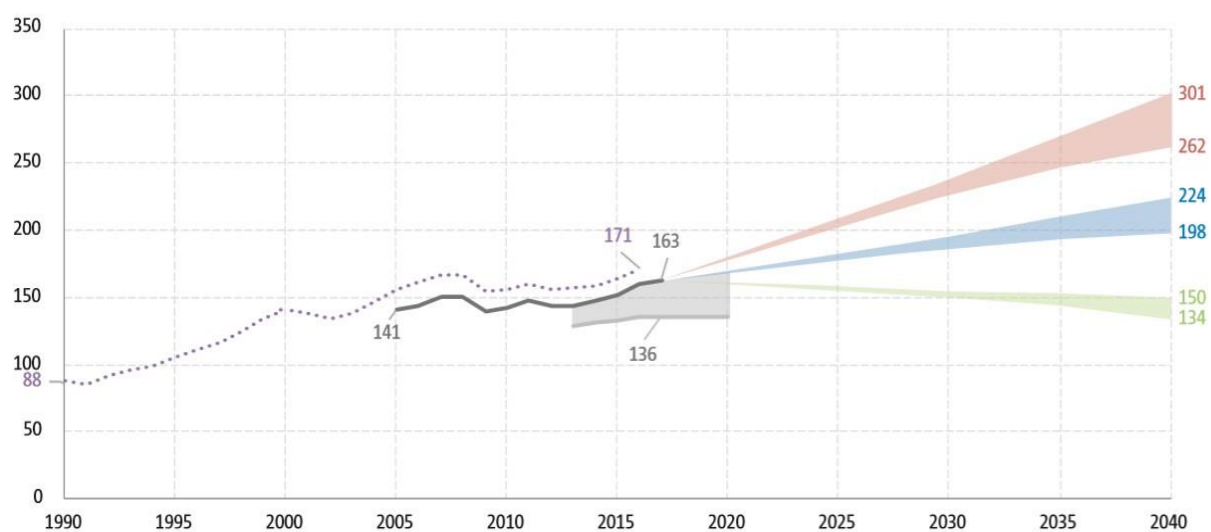
Figure 2: Projected CO 2 emission from European aviation in Mt till 2040 (EU 2019).
